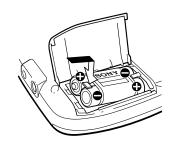
**3** Connect the AC power adaptor. The indication "CHG" lights up and the 'number 1" shifts position in succession until the battery is fully charged. Charging time is about 2 hours for BP-DM10 and 3.5 hours for BP-DM20.
